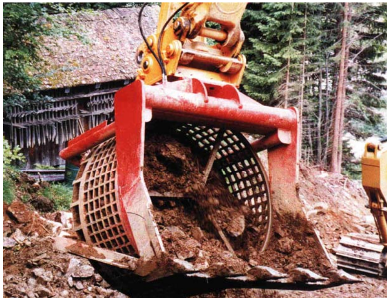
Screening adapter (for recycled material)
