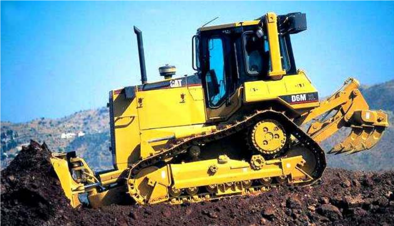
Bulldozer equipped with ripper attachment
