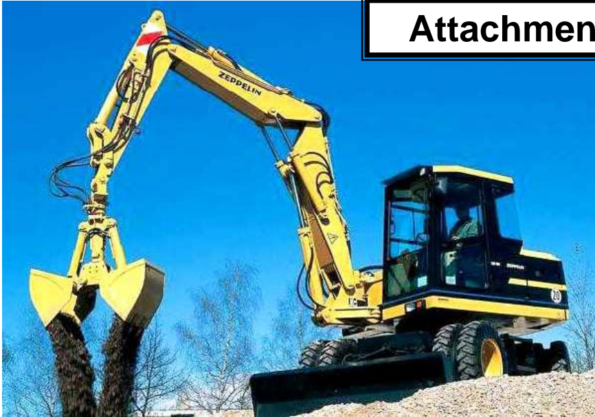
Clamshell bucket (for granular material)
